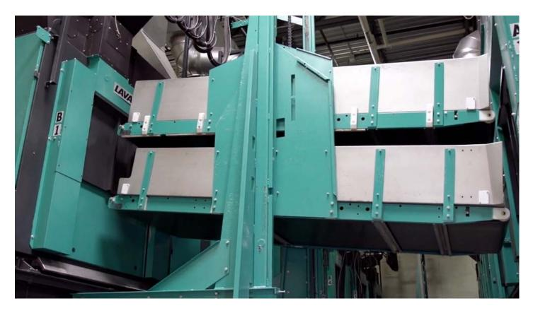
also have two Lavatec washer extractors with standalone dryers. Lavatec conveyors link system components, and move goods from dryers into finishing, and a Lavatec rail system gets the laundering process literally up and running in soil-sort, expediting overhead transfer of loads to each washer.
