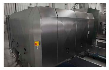
Variable discharge option enables Metropolitan Detroit Area Hospital Services, Inc. (MDAHS) to direct goods to either the extraction presses or - in the case of surgical garments and other items with micro denier fabrics - to the centrifuge, which provides gentler spin extraction in order to preserve linen integrity. System equipment is manufactured by Lavatec Laundry Technology (LLT).
