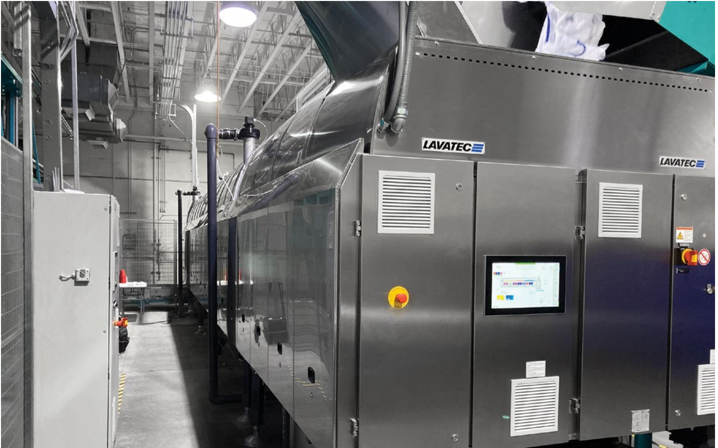
The shuttle system feeds the new LAVATEC tunnel, which is helping Southern Oregon Linen Service reduce their water usage by an average of 30,000 gallons a day.
